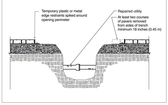
Figure 8. T-shaped cross section of the excavated opening
