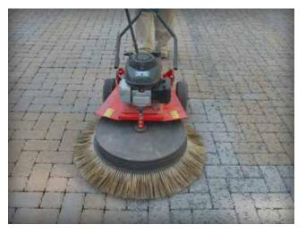
Figure 16. Rotary brushes increase cleaning efficiencies.
