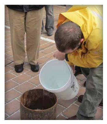
Figure 13. ASTM C1781: pouring the wanter into a 12 in. (300 mm) inside diameter ring set on plumber's putty.
