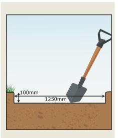
2. Dig to a depth of approximately 100mm. Remove all roots and plant matter within the perimeter.
