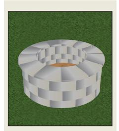
8. Finally, fill the completed fire pit to the desired level with river sand - normally level. Up to 150mm (one course height) from the top.
