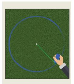
1. Use rods and string to demarcate a radius of 625mm, where you would like to place the fire pit. This will demarcate the outer perimeter of the fire pit. The diameter will be 1250mm.
