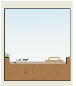
3. Add ±40mm of moist river sand where the blocks are to be placed. Even out the river sand and ensure that it is level.
