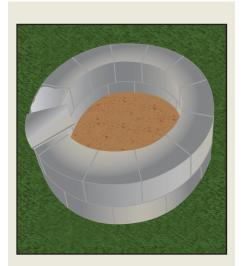
7. Place the coping over the last block layer, again with each centre over the joint below; ensuring that the copings fit together neatly. Remove the copings one-by-one and apply the 3:1 mix of building sand and cement to the last layer of blocks. Place the coping down again, and apply pressure; ensuring the coping is level.
