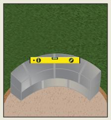
4. Place blocks tightly in a circle. Start by completing the first layer and then level the blocks with a spirit level.
