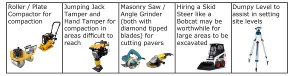
The following specialist tools are recommended to make the installation of paving safer, easier and more accurate. They are imported from *Probst*, in Germany, and available in South Africa from *Cretesol*.
